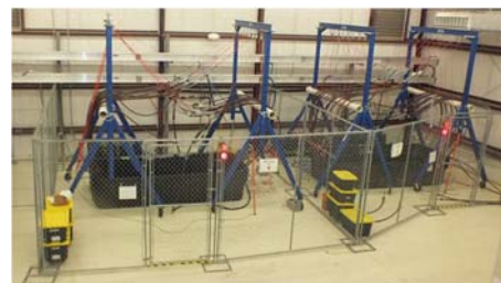
Samples under test, joints were submerged in the tanks (~1 ft depth) with spacing off the bottom of the tank and between each other.
