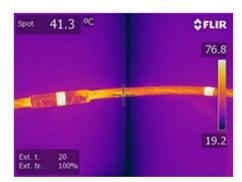
Direct temperature measurements are easier and more reliable than IR for assessing the absolute temperature of a connector. Sufficient current is needed at the time of measurement just as for IR imaging. This hotstick-based technique must be in contact with the line for several seconds to obtain an accurate temperature measurement.
