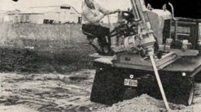
Jaques TJ-254 digging at 30-degree angle. Operates at up to 45 degrees.
