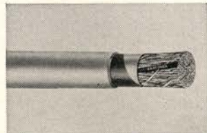
Anaconda Type PL Paper-Lead Cable (No. 19, 22, 24 & 26 Awg). Single-paper-tape insulated telephone cable, paper core covering over assembled pairs; antimony-lead sheath overall.
