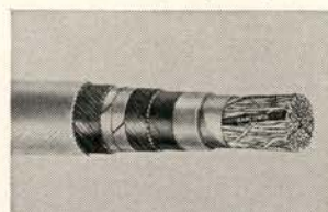
Anaconda Type PLP Paper-Lead Polyethylene Protected Cable (No. 19, 22, 24 & 26 Awg). Paper insulated, paper core covering, assembled pairs; antimony-lead sheath, polyethylene jacket.
