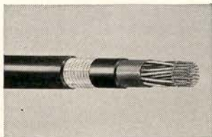
Anaconda Type PCP Direct-Burial Cable (No. 19, 22 & 24 Awg). Polyethylene insulated; full color code; polyethylene belt; 5-mil longitudinal copper shield; polyethylene jacket.
