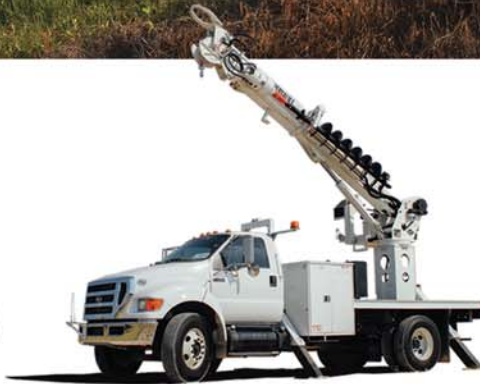
TMD DIGGER DERRICK
