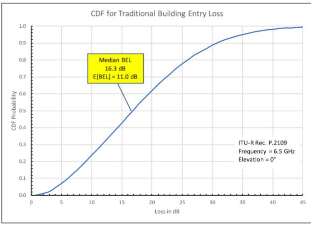
Figure 10 Cumulative Probability Distribution of Building Entry Loss
