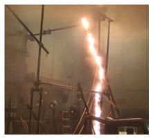
current carrying capability should a fault occur during the time that they are attached to a utility system. In this project, NEETRAC will perform fault tests on various aged TPG assemblies to gather data on their performance. These results will be compared to results from new TPG assemblies tested in a previous NEETRAC Baseline project to establish whether or not their fault current carrying performance deteriorates as they are used in service.
