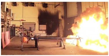
for directionally bored systems that do not utilize concrete or grout. The purpose of this project was to conduct tests to determine if an arcing fault in one cable / conduit assembly can easily propagate through to adjacent conduits and cables. High power fault tests were conducted to determine if directionally drilled cable systems could meet the NESC requirement.
