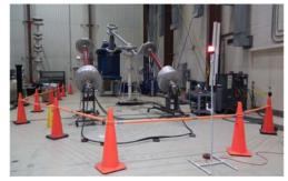
aging qualification results and showed that the two underground system components age differently – at least for the joint type evaluated. This led the NEETRAC Management Board to consider further tests on other joint designs to gain a more in-depth understanding of joint performance under long term accelerated aging test conditions (project #19-091).
