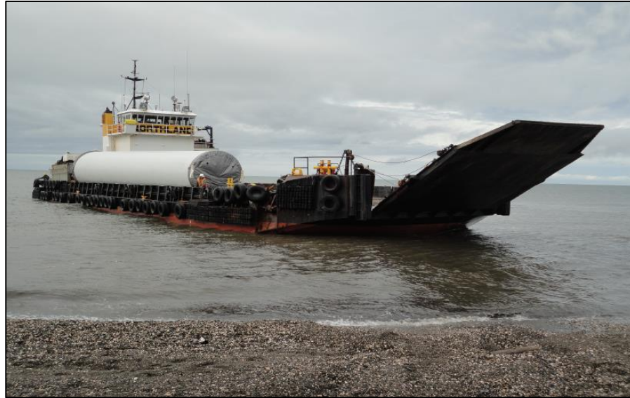
Figure 4. Barge transporting wind turbine tower segment. Courtesy of Kotzebue Electric Association.
