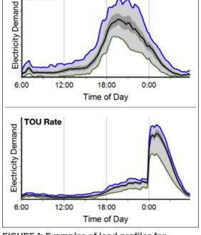
FIGURE 1: Examples of load profiles for uncontrolled EV charging (top) and indirectly controlled charging through TOU rates with off-peak hours from midnight to 6 am (bottom). Figure modified from The EV Project (2013).
