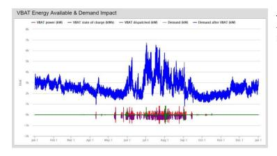
This graph displays the hourly demand, virtual battery state of charge, and the impact of the virtual battery on the demand.
