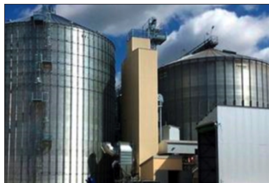
FIGURE 7: Example of a Tower Style Radio Wave Grain Dryer (Source: DryMax website )
