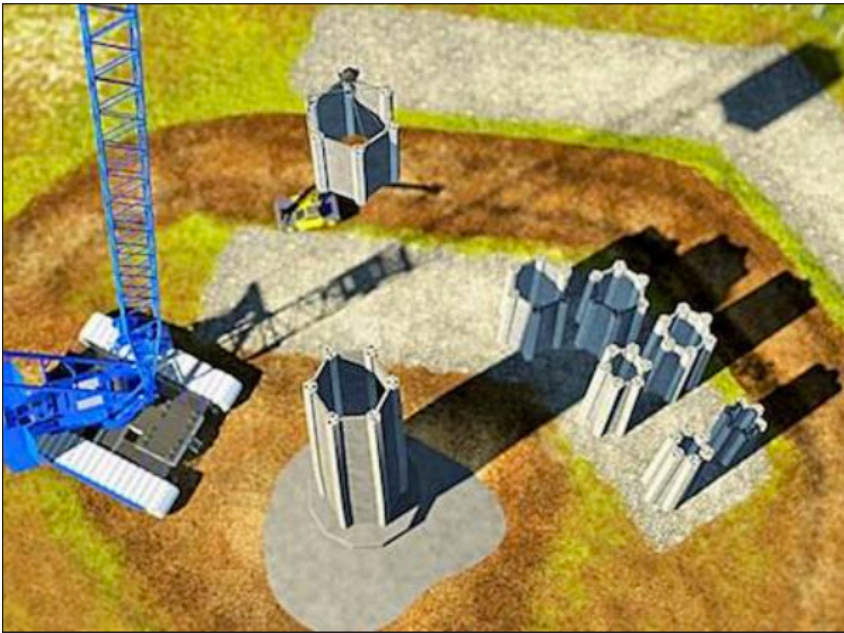
FIGURE 3: Image showing how Hexcrete cells can be assembled on-site and stacked to 140 meters high by a crane. Image courtesy of Sri Sritharan/Iowa State University
