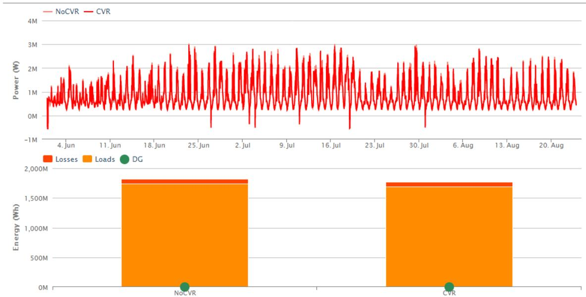
Figure 5. Three-Month Dynamic Powerflow Simulation—Powerflow across the Substation, and Loads and Losses Breakdown
