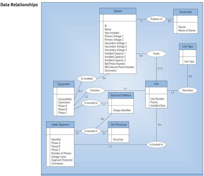
FIGURE 2.2: Electric Network Conceptual Representation in the GIS
