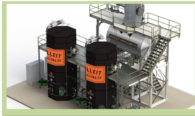
Figure 1.3: Rendering of electrode boilers to be installed at the Lebanon, Kentucky distillery. Courtesy of Precision Boiler and Diageo
