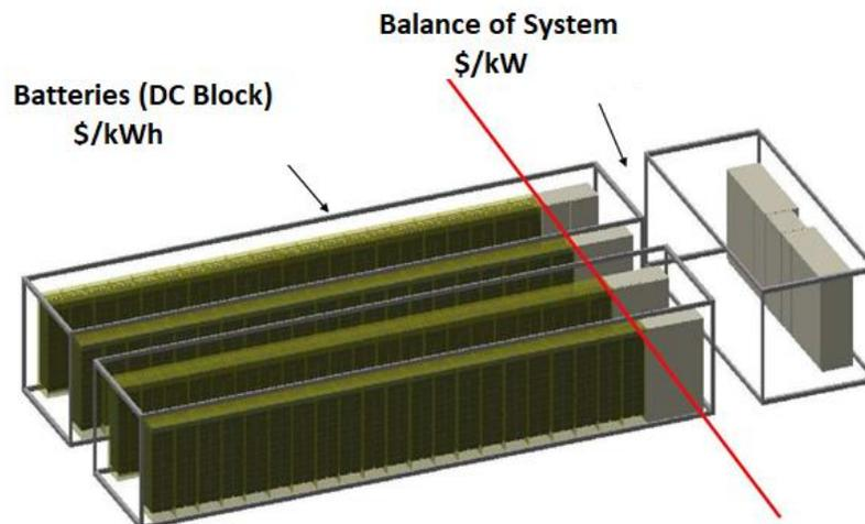
**FIGURE 3.1 – Cost Components of a BESS**
