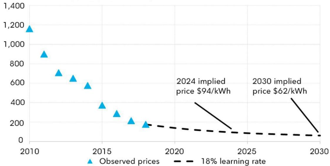
**FIGURE 3.4 – Li-ion Battery Module Costs Trend & Outlook (2018 \$/kWh)**
