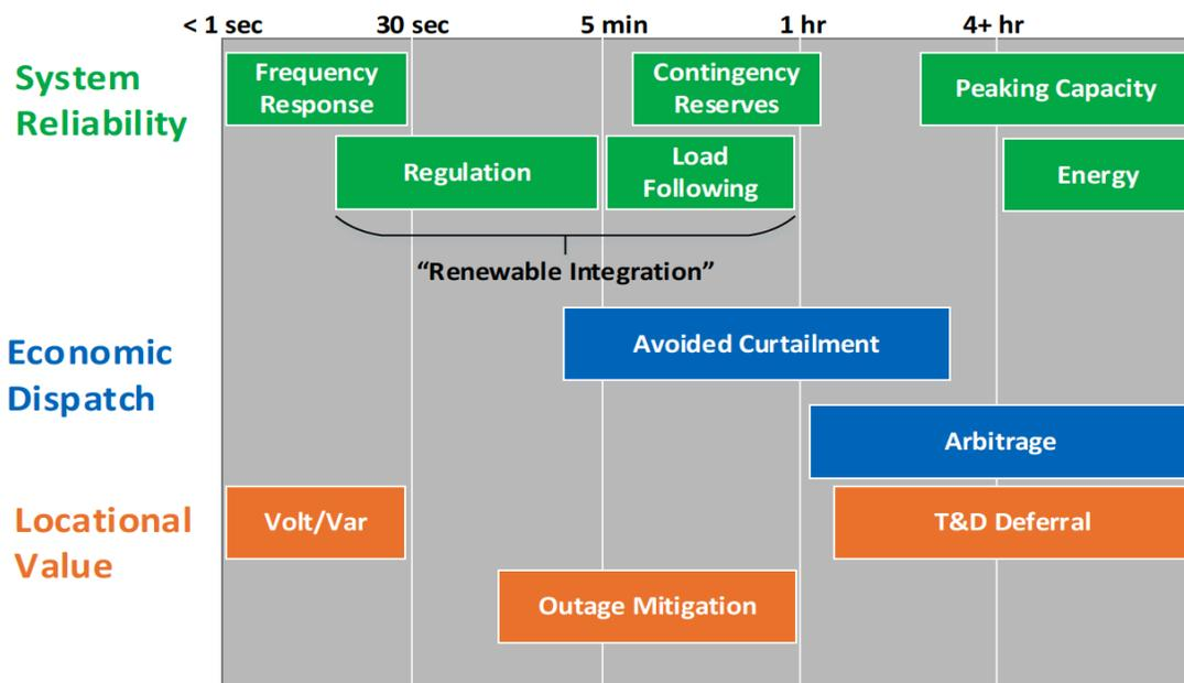
**FIGURE 3.8 – Use Case Applications for Batteries**
