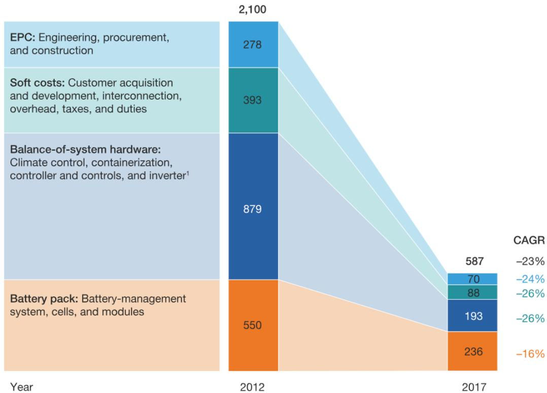
**FIGURE 3.5 – Cost Breakdown of a 1 MWh BESS (2017 \$/kWh)**
