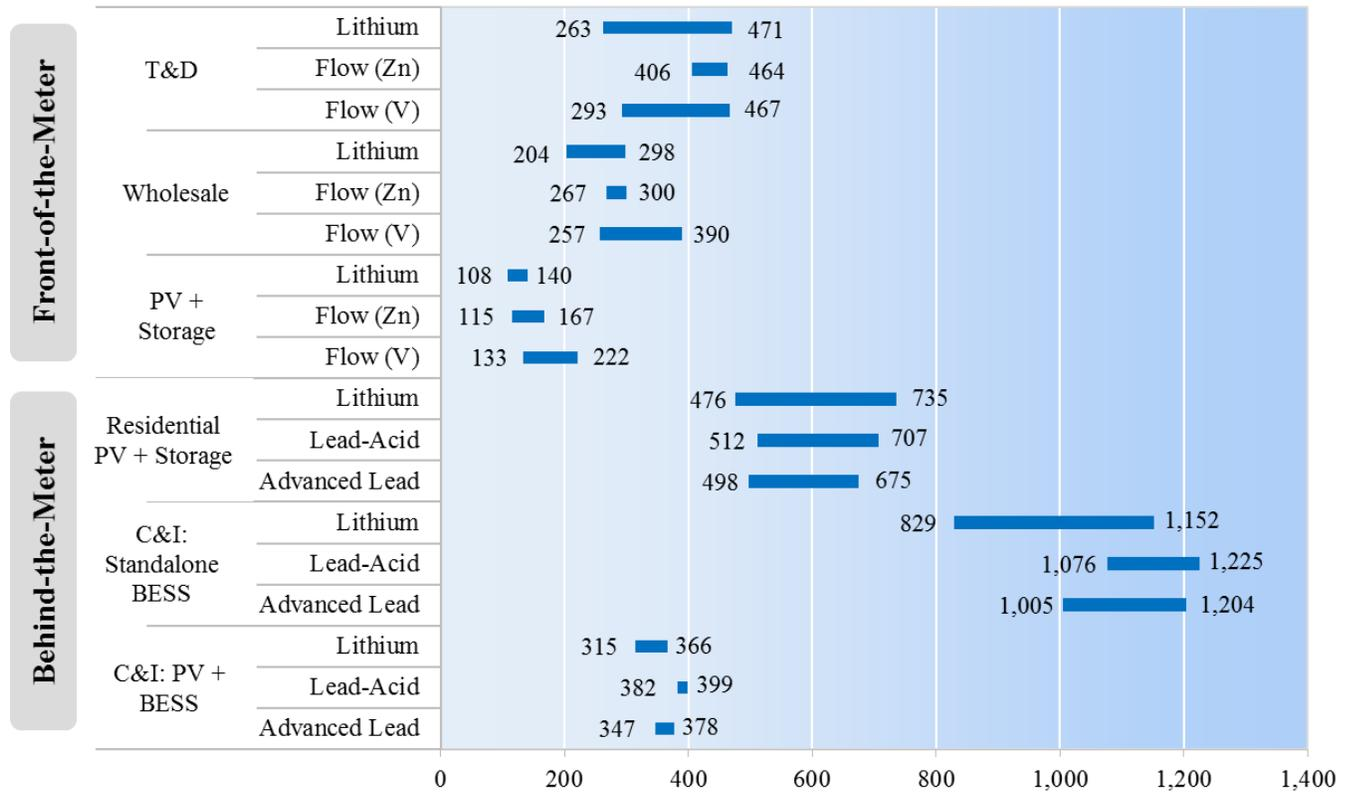
**FIGURE 3.7 – Comparison of Unsubsidized LCOS (\$/MWh)**
