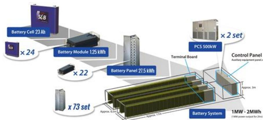
**FIGURE 3.3 – Relationship Between Battery Cells, Modules and Panels**
