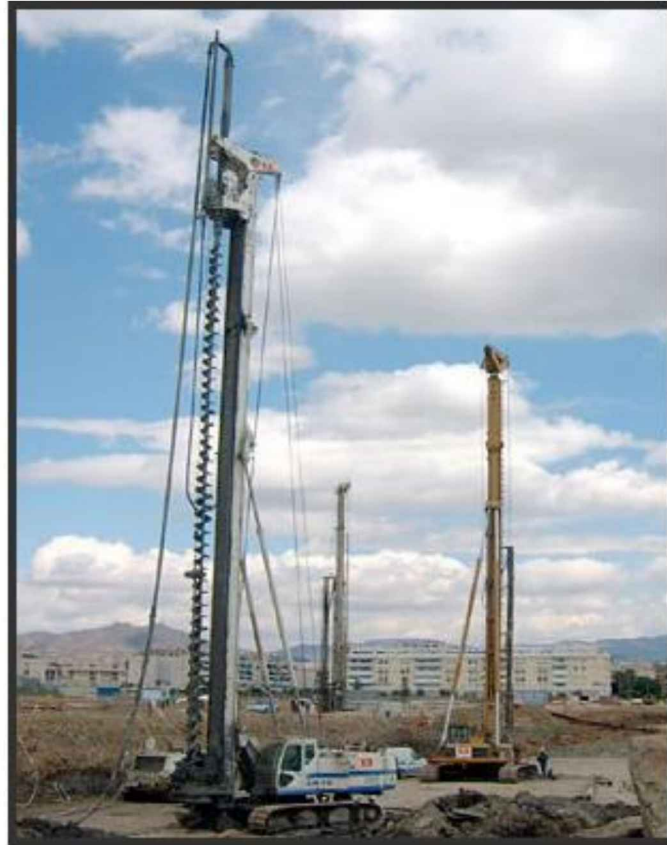
Figure 6-31: Soilmec Hydraulic CFA Rig with Kelly-bar Extension (Brown et al., 2007).
