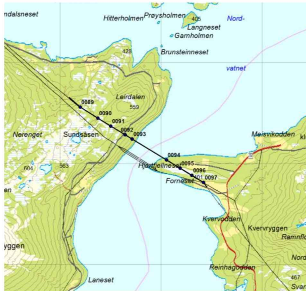
Figure 5-1: Line route map showing the sections affected by the wet snow icing.
