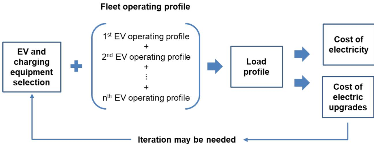
In order to estimate the costs of electricity and electric infrastructure upgrades associated with a fleet electrification project, a fleet customer first will need to determine how its EVs will charge. Figure 7 illustrates how to step through this process, which is described in more detail below:
