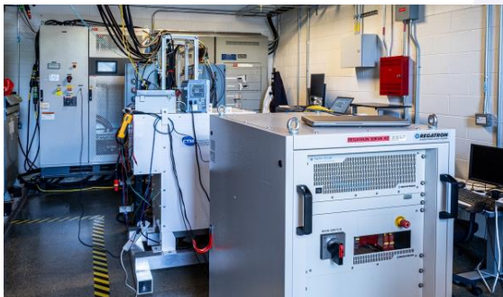
Photo by NREL. NREL-owned ABB FC inverter
